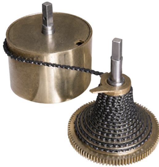
Fig. 3. A clock fusee chain.
