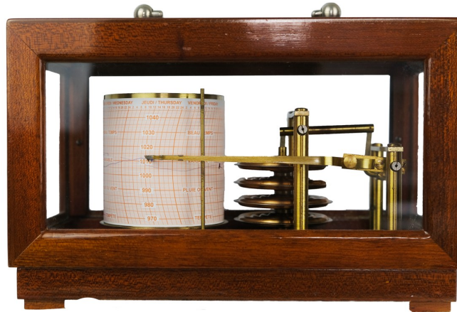
A barograph with a stack of individual capsules.
